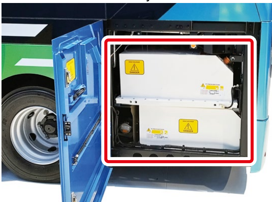
Left hand rear side battery locations
